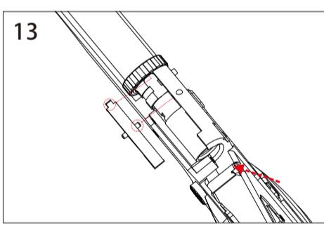
13. Replace the hop-up pressure plate, the lever should located inside the hop-up adjust knob.
