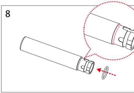
8. Replace the o-ring from the out barrel to the thread barrel.
