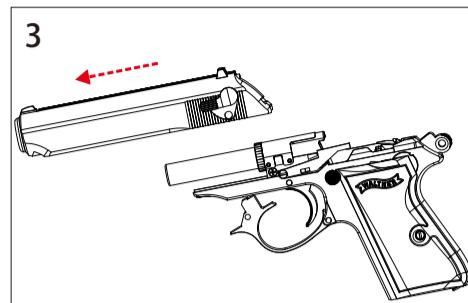
3. Remove the slide, and the recoil spring will be removed together.
