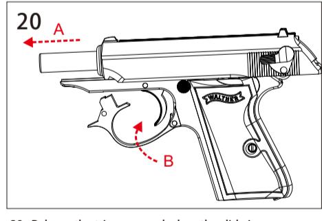
20. Release the trigger guard when the slide is already lined back up with the frame.
