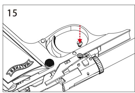
15. Replace the slide catch and the spring, and the spring should be in the groove.
