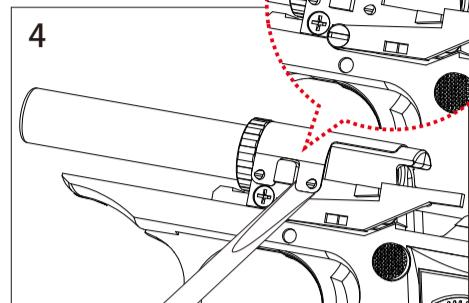
4. Use the flat head screwdriver to pry open and remove the dummy chamber.
