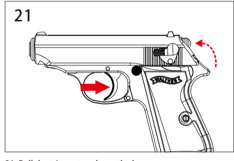
21. Pull the trigger to release the hammer.
