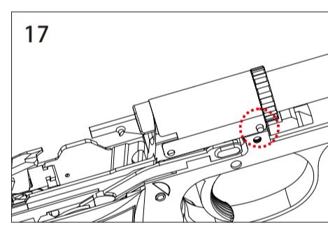
17. Replace the dummy chamber from the right side.
