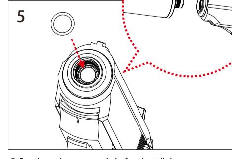
5. Put the o-ring on muzzle before install the suppressor.
