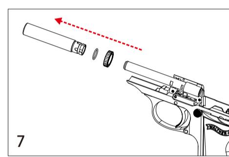
7. Take down the out barrel, out barrel o-ring, hop-up adjust knob and inner barrel set.
