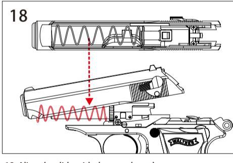
18. Align the slide with the muzzle and make sure the recoil spring is on barrel.
