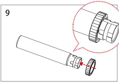
9. Install the Hop-up adjust knob on the barrel.
