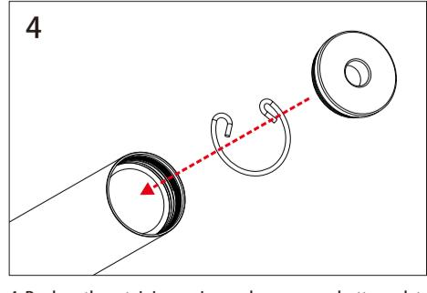
4. Replace the retaining spring and suppressor bottom plate.
