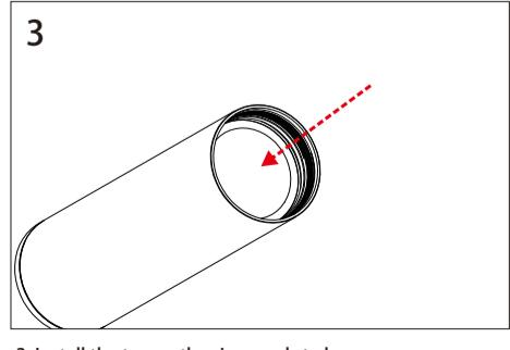
3. Install the tracer, the size needs to be within 50mm in height and 26mm in diameter.
