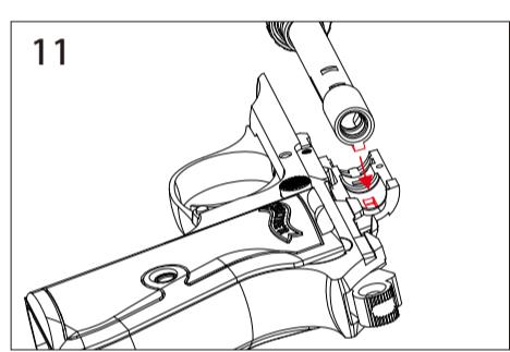
11. Replace all the barrel parts into the hop-up base.
