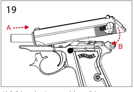
19. Pull down the trigger guard then pull the slide back to the bottom and lift down it.
