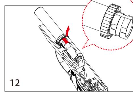
12. Make sure the flat surface is on the top of the barrel.
