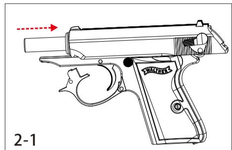
2. Pull the slide back to the bottom and lift up it.
