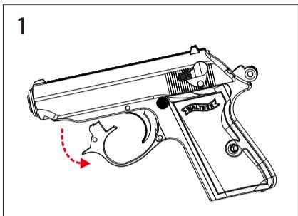
1. Take down the magazine and pull down the trigger guard.
