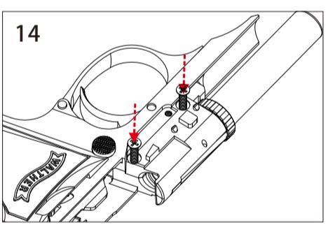
14. Replace the hop-up left side and screw on.
