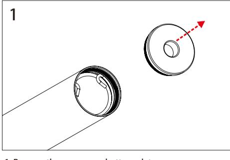
1. Remove the suppressor bottom plate.
